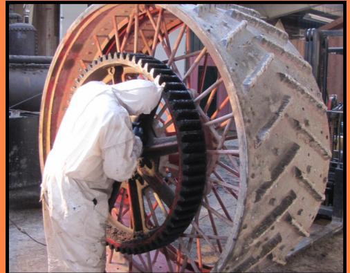
Gregg Crew removes years of grease and grime from the gear of a back wheel.
