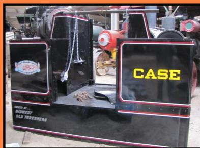
Left: The boiler is ready for paint. Above: Rebuilt bunkers wait to be mounted on the 110.
